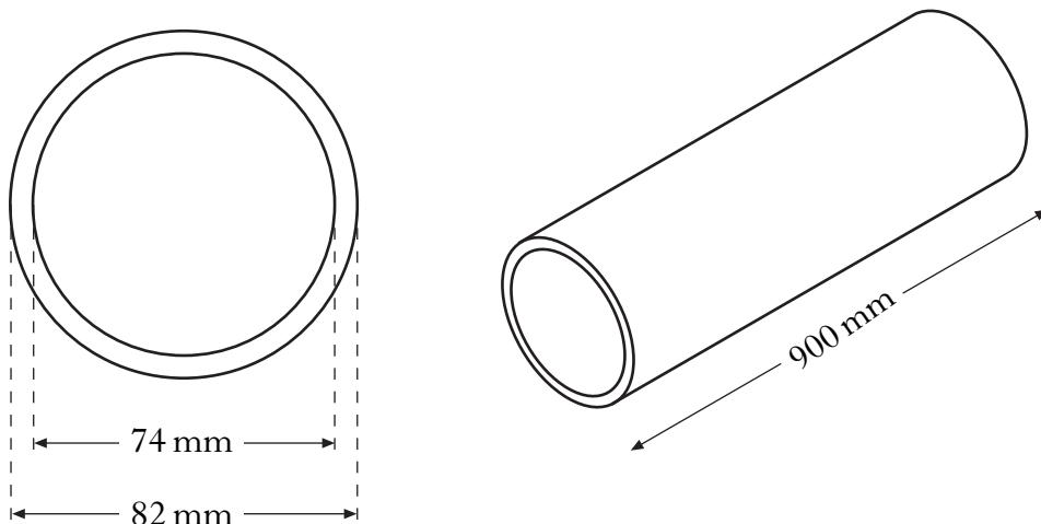
The inner diameter is 74 millimetres.
